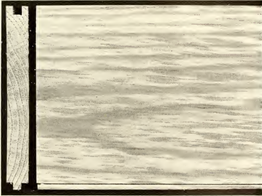
FIGURE 2-95.—Planed southern yellow pine board showing typical sap stain.
